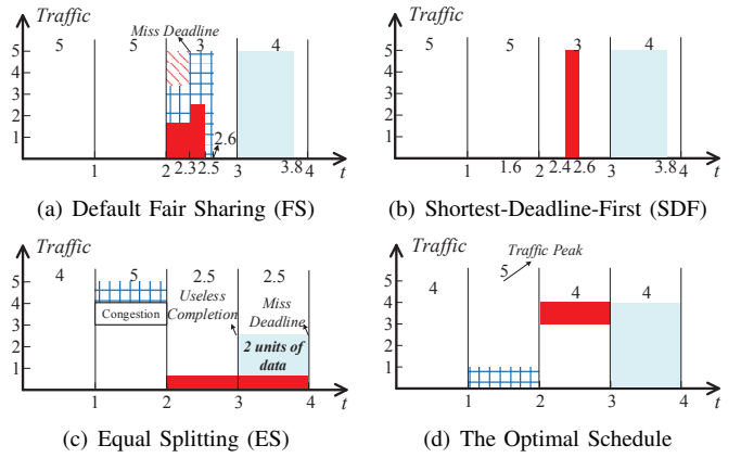
Fig. 2. The billed bandwidth usage under the 75-th percentile charging model for (a) FS is 5; (b) SDF is 5; (c) ES is 4; (d) optimal schedule is 4. Both FS and ES miss some flows’ deadlines, while SDF and optimal schedule accommodates all flows with deadlines guaranteed. The bandwidth consumption on each time slot is listed in the top of each sub-figure.
