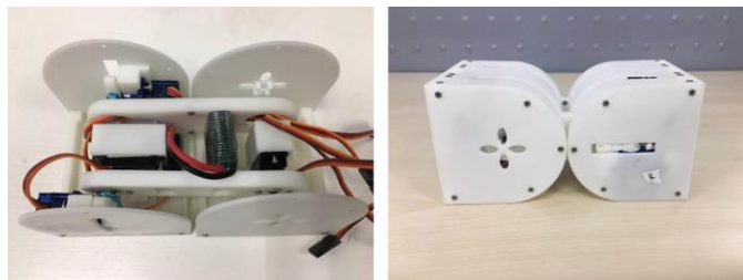
Fig. 1. The physical prototype of the EasySRRobot. The interior structure (left) and the outmost shape (right) of the module.
