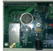
Fig. 6: The prototype of the wireless gas leak detection sensor node
