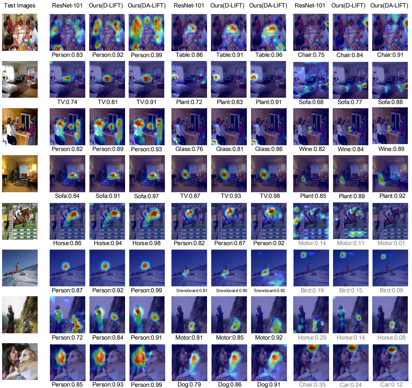
Fig. 7. Visualization results of our model with Grad-CAM [50]. We compare the visualization results of Deep-Attention-LIFT (DA-LIFT) with Deep-LIFT (D-LIFT) and the baseline (ResNet-101) in the target layer of deep attention LIFT map, deep LIFT map and “conv5_x”. The sigmoid scores for top-3 highest-ranked target classes are also shown for each test image. The labels in black and gray indicate positive and negative classes of the image respectively.
